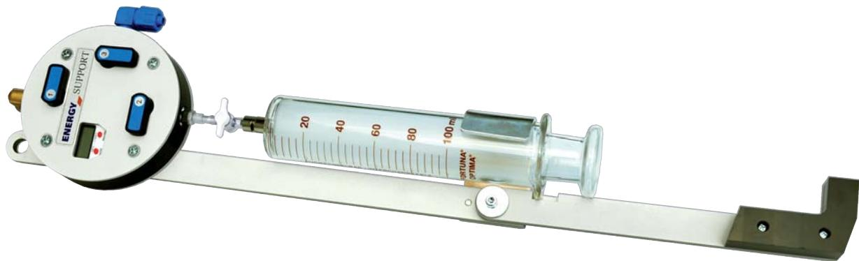
The sampling syringes (100 ml - fully made of glass) are gas-tight and equipped with a special valve. Together with a flexible PFT tube, the syringes can be directly connected to the oil-sampling flange of the transformer.
